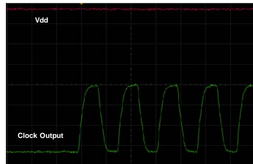
Figure 17. Startup Waveform vs. Vdd (Zoomed-in View of Figure 16)
